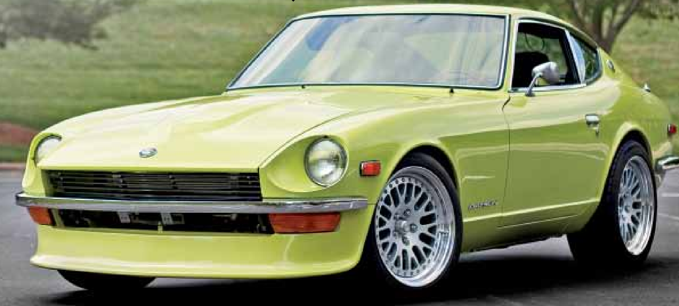
Exterior Miller Brothers Hot Rod Barn complete restoration, modified bumpers (converted from 3-piece to 1-piece & moved 0.50" closer to the body)
