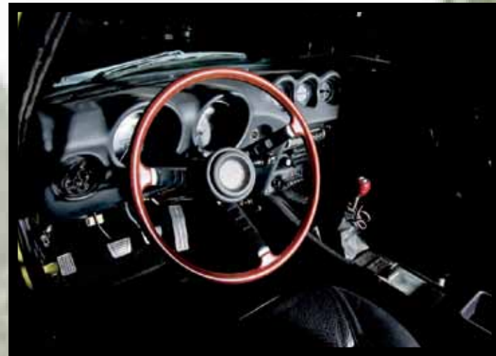
Interior Miller Brothers Hot Rod Barn complete restoration (including brand-new OE dash); Classic Datsun Motorsports restored steering wheel & horn button; National Speed center console "power switch"; Wilwood brake proportioning valve
